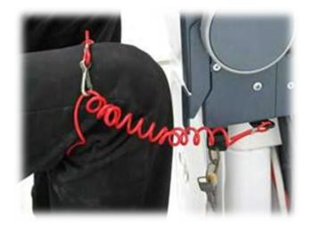
Kill cords should be protected from the elements. Over time extremes of temperature and UV light will harm the lanyard. Kill cords may become stretched or brittle if stored open to the elements. Monitor the kill cord for signs of wear, rust and reduced elasticity (the kill cord should not droop excessively) and replace it in good time.
