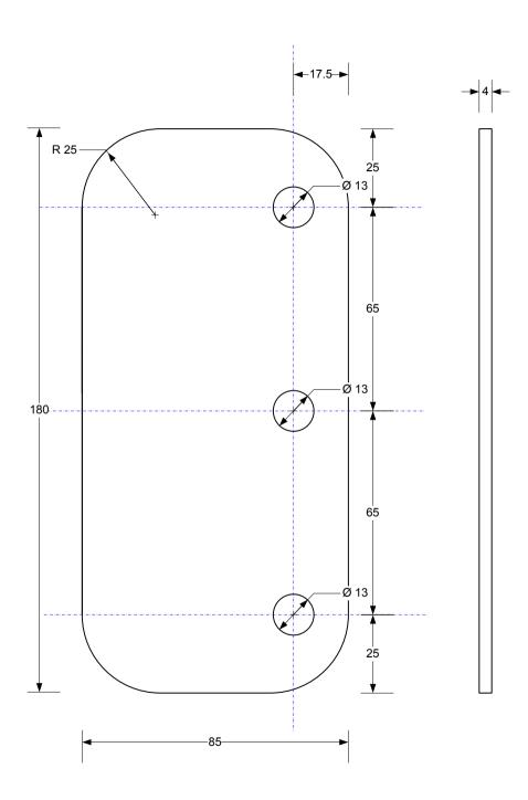
Detail D: Forward Support Arm Attachment Plate
