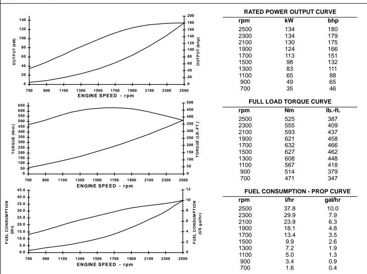
Rating Conditions: Ratings are based upon ISO 8665 and SAE J1228 reference conditions; air pressure of 100 kPa [29.612 in. Hg], air temperature 25°C [77°F], and 30% relative humidity. Power is rated in accordance with IMCI procedures. Member NMMA.
