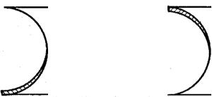
sander chamfer off the top rear section and bottom front section of the edge until the whole width sits flat against the tube.
